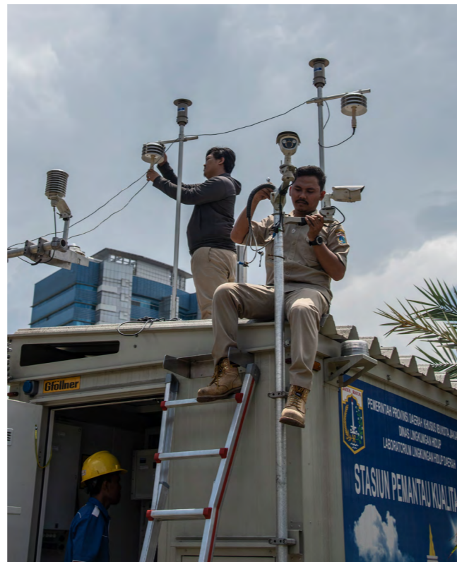
Above, Staff from the Environmental Agency of Jakarta carry out routine maintenance on their Air Quality Monitors. Photo: Vital Strategies, 2019.
